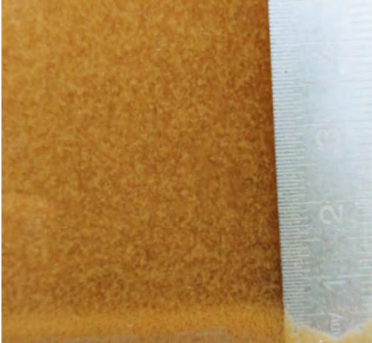
Fig. S5. Plume aggregates during deposition (0.6 mm: compaction area ; 6 - > 40 mm: agglomeration) in the flume
