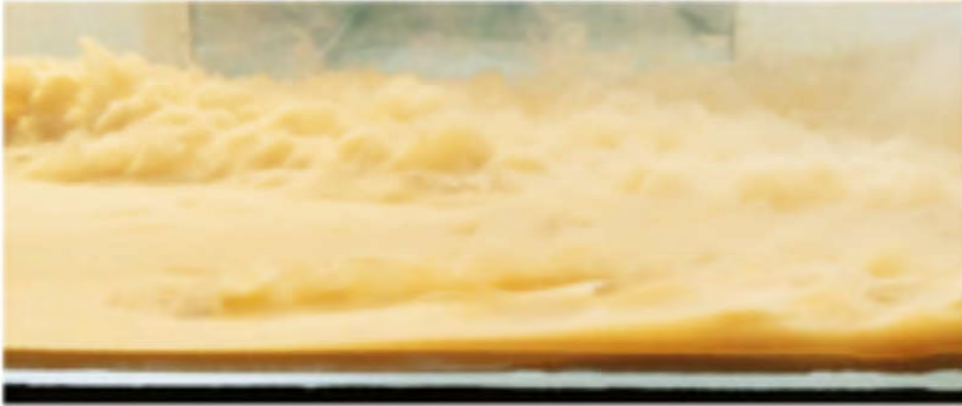
Fig. S1. Incoming gravity flow under 0.1 G conditions in the seawater flume
