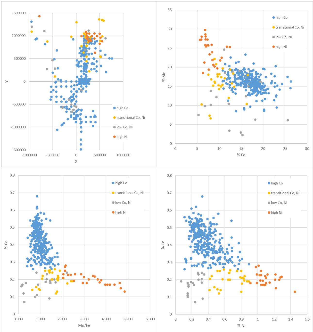
Figure 4-25: Spatial distribution and grade relationships between nodule grade types. Coordinates are from a custom Lambert azimuthal equal-area projection centred on 16°S and 161°W.
