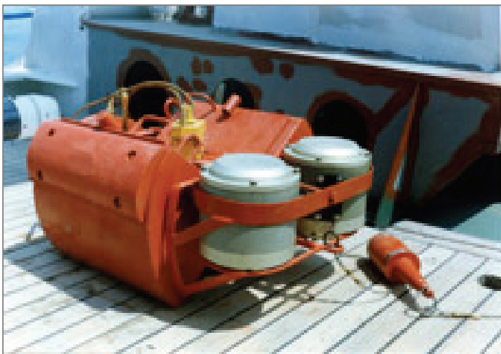
Figure 11.1 Ocean-0.25 Grab Sampler (Yubko, 2012)
