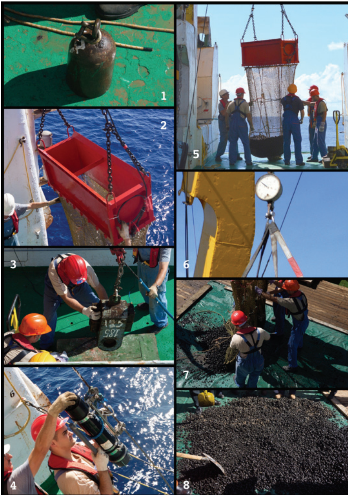
Figure 9.33 Operations and details of the YMG Galatea-trawl dredge
