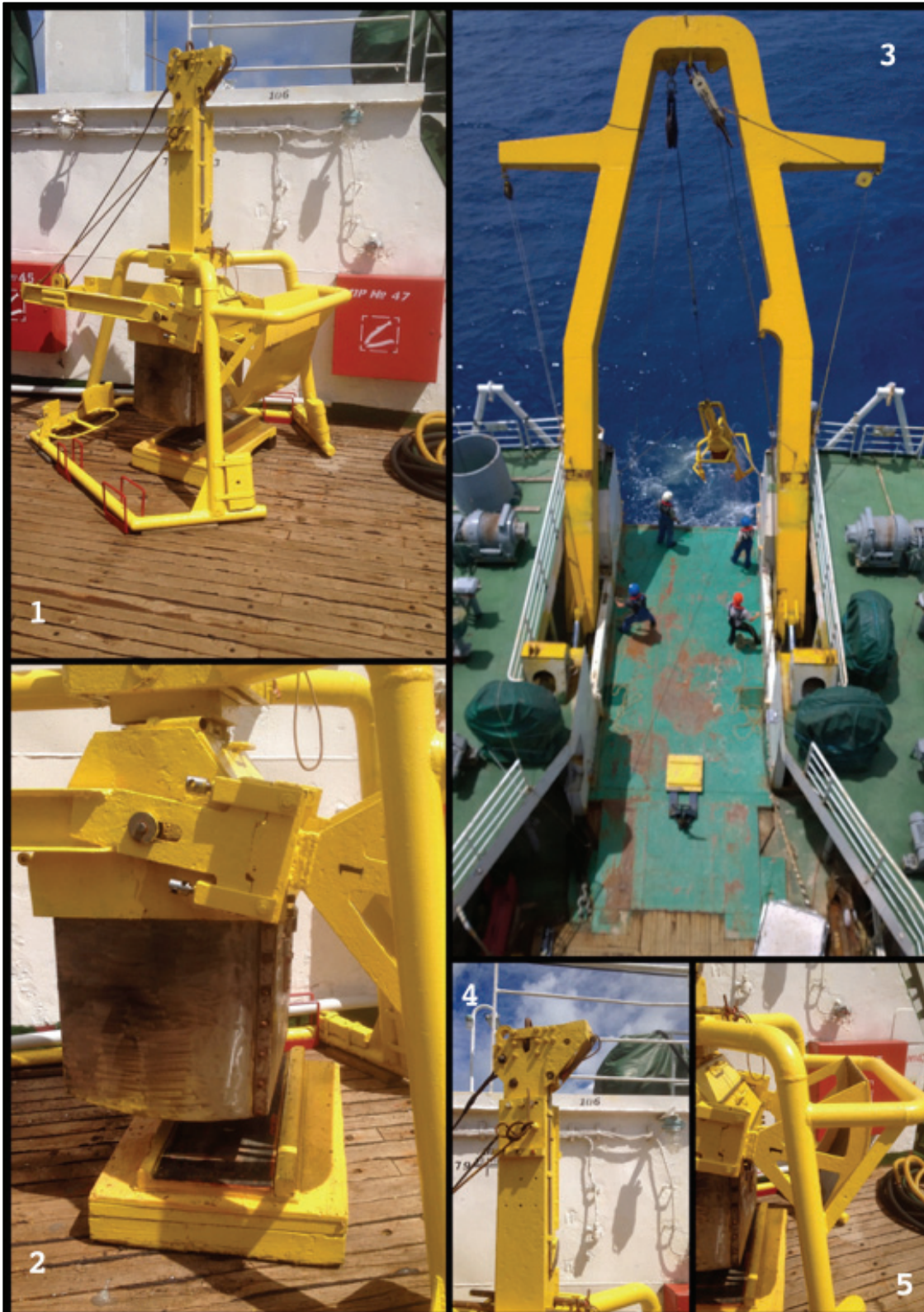
Figure 9.15 Details and recovery of the YMG box-corer
