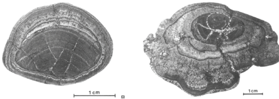
Figure 8.1 Sections through a S-type Nodule (left) and a R-type Nodule with a S-type core (right)
