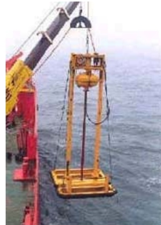
Figure 7.6. HPC Vibrocore seabed sampling.
