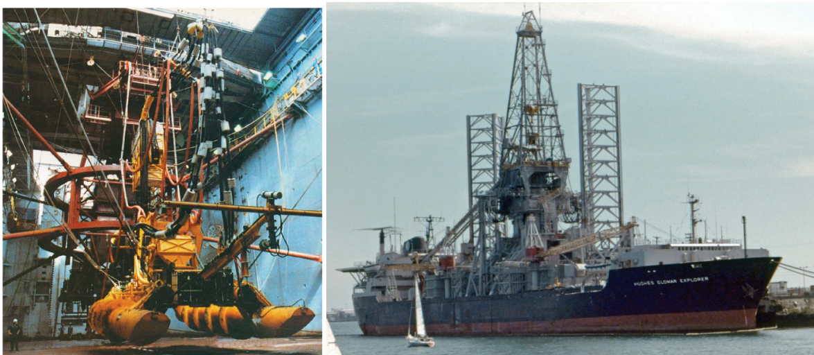
Figure 6.20 OMCO Screw-drive collector and pilot mining vessel, the USNS Hughes Glomar Explorer
