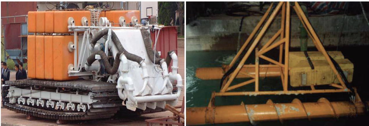
Figure 6.26 Chinese pilot scale tracked and test screw-drive subsea vehicles
