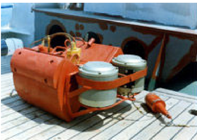
Figure 11-1: Ocean-0.25 Grab Sampler (Yubko, 2012).
